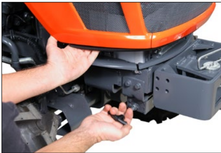
Bonnet access without tool for the EK1-261 or with the tool inside the toolbox for the others.
