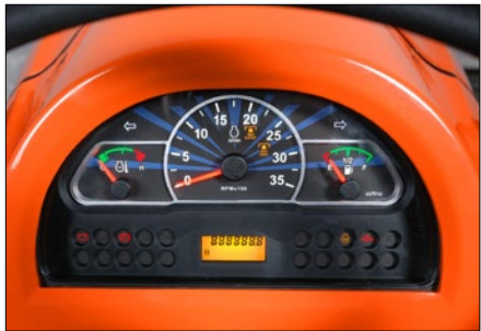
A sensor on the dashboard indicates when the air filter needs cleaning, simplifying maintenance.
